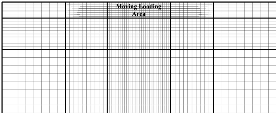
Figure 37. Surface layer mesh in plan view.
